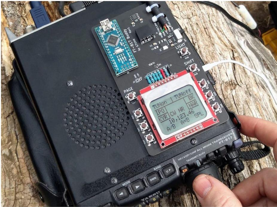
Last month, inspiration struck and I thought I could cobble together a small microcontroller and a little OLED display with some buttons to provide some extra soft-keys for the radio using the CAT serial port.
