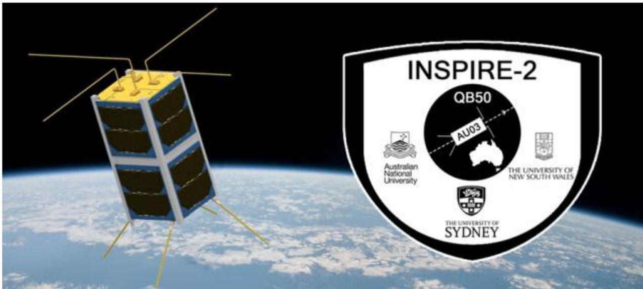
It was placed in orbit from the International Space Station in late May. The deployment was successful; however there were no signs of life when the ground stations started looking for it. The engineering group quickly tested various scenarios on the engineering model only to come to the conclusion that, due to the extended delay in the deployment, the satellite's battery was likely to be depleted and the satellite was trapped in an endless loop, trying to deploy its antenna.
